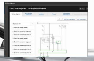
The guided diagnosis allows identifying, locating and solving any errors in the electrical system and components through a procedure integrated in the IDC5 diagnostic software.
